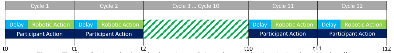
Figure 6. Timeline of cycles and actions taken by each agent. Robot actions are delayed randomly to lessen learning effects
