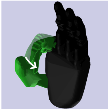
Figure 8.9: Example for how the joint angles were biased for hand calibration. Bias effect is exaggerated for clarity. [Best viewed in color.]
