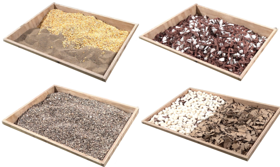
Figure 6.5: Example terrains illustrating different compositions, materials, and topography. Top left: Partition of Sand and Corn. Top right: Mixture of Mulch and Gravel. Bottom left: Single of Pebbles. Bottom right: Layer of Shredded Cardboard (right), Packing Peanuts (left, top layer), and Slates (left, bottom layer).
