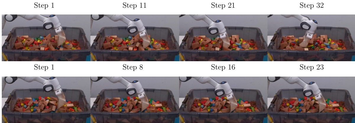
Figure 7.7: The top and bottom rows show two example trajectories executed with MCTS, k = 5 , tracking the deep trajectory. In the top row, a few objects are successfully excavated, while the excavation is aborted due to large contact forces in the bottom row.
