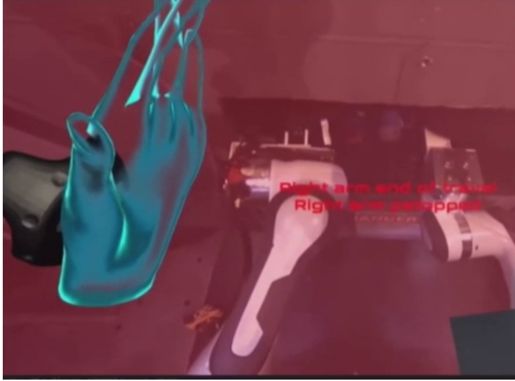
Figure 8.13: The operator’s view after AVATRINA’s right arm engaged mechanical brakes in response to excessive force. [Best viewed in color.]
