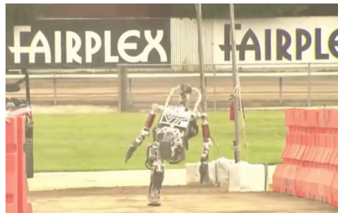
(b) ESCHER robot falling failure
