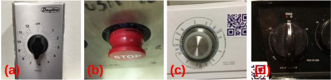
Figure 6.11: Four button types that SwitchIt failed to activate: (a) An old-style timer, (2) An elevator pull button, (3) A washer control button, (4) A turn knob on oven.
