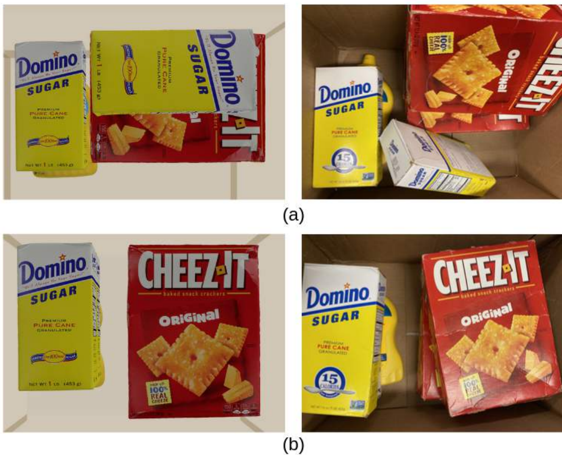
Figure 5.5: Conservative geometry margins reduce inadvertent collisions. (a) A non-conservative plan (left) causes a failure during the execution of the plan (right). Specifically, the shifted cracker box caused a failure and crash of the sugar item planned on top of it. (b) A conservative plan with \delta = 1 cm margin. During execution, all items are placed within the container without causing an inadvertent collision.
