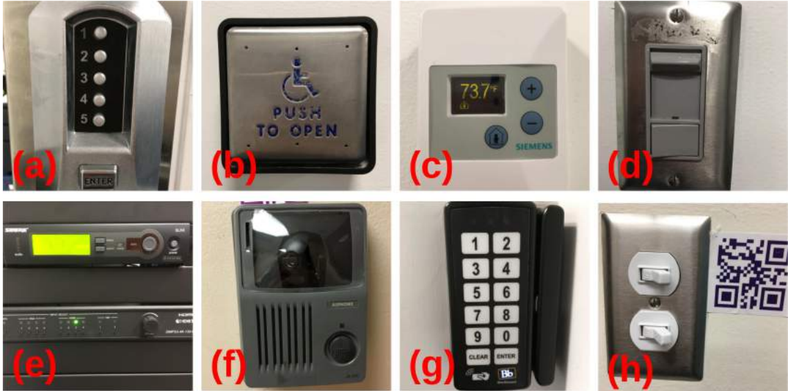
Figure 6.10: A selection of button panels that SwitchIt succeeded in activating: (a) Door passcode, (b) Disabled door exit, (c) Thermostat buttons, (d) Switch with dimmer, (e) Office stereo control, (f) Security door entrance, (g) Electronic keypad, (h) Light switch
