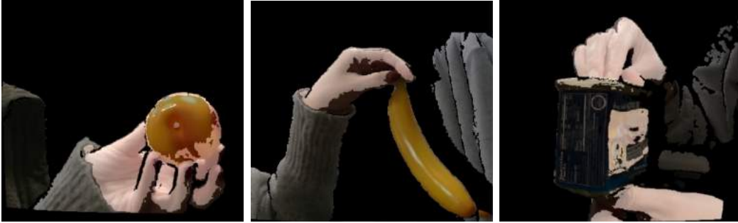
Figure 4.2: Skin regions identified by skin-pixel based segmentation described in [VSA03]. This method cannot detect shaded areas of hand as well as accessories on hand (jewelry, nail polish, etc.). It also falsely includes object regions with colors close to human hands.
