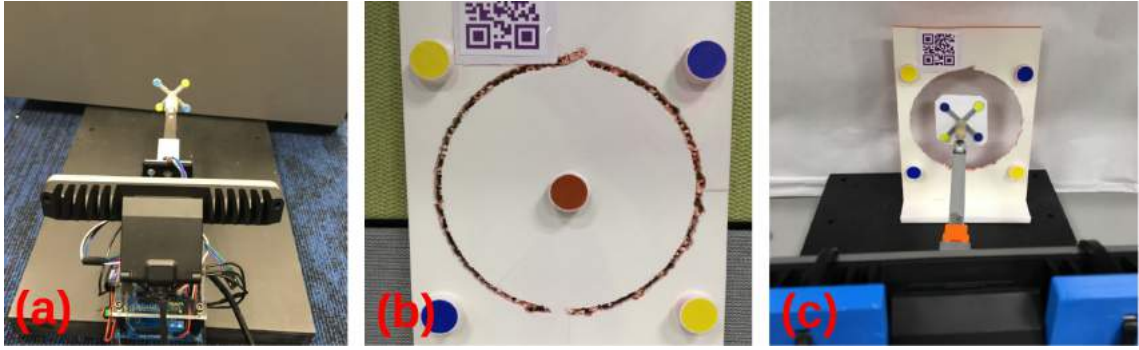
Figure 6.7: The above apparatus is used for testing the accuracy of the system: (a) Robot and camera are calibrated using a cross marker, (b) Center button is located at the intersection of opposing diagonal circles, (c) Center plate is removed during the test to not interfere with tip motion.
