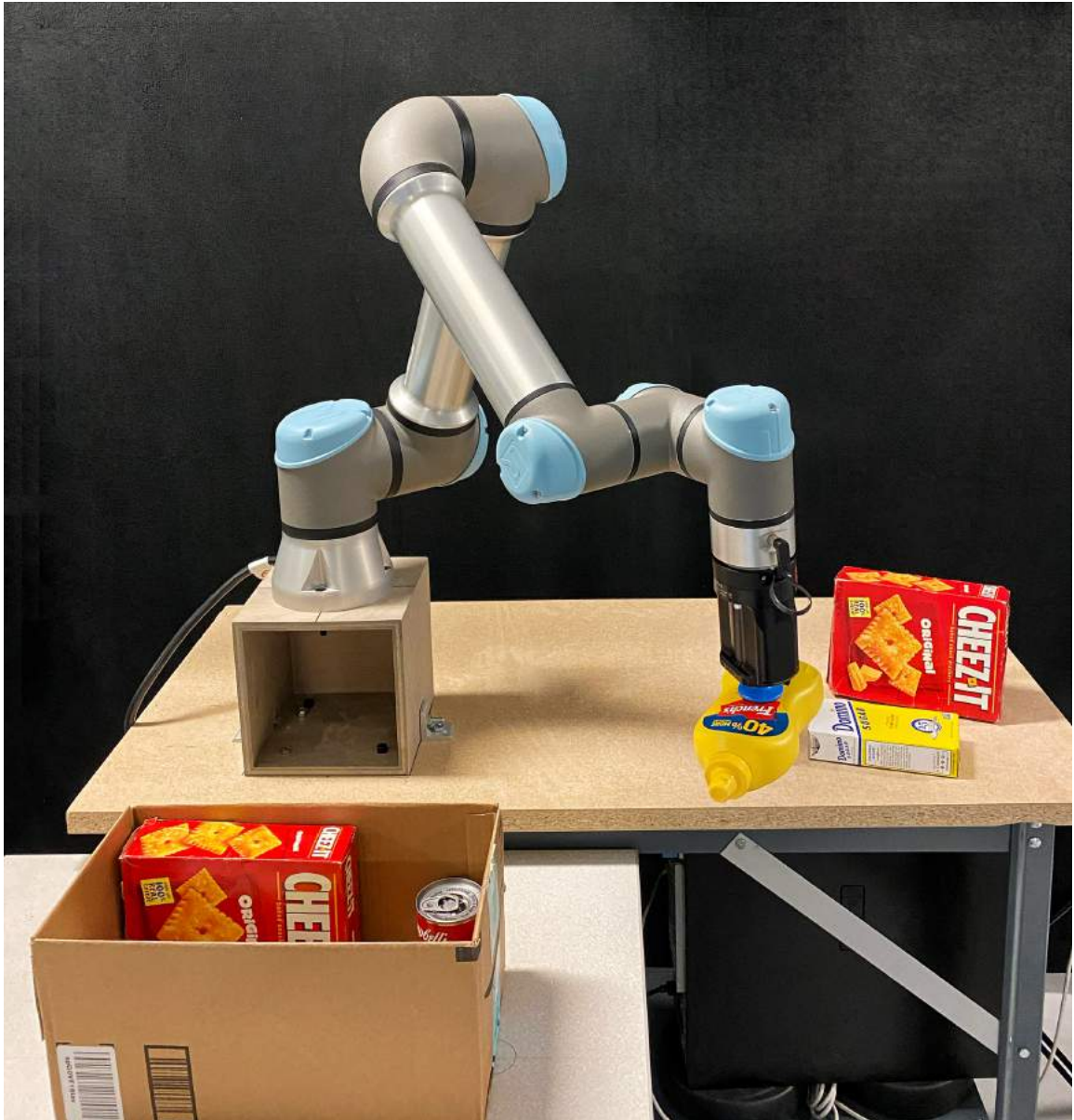
Figure 5.1: The experimental packing setup consists of a UR5 robot equipped with E-pick suction gripper, and overhead cameras (not pictured). Errors from pose recognition, camera-robot calibration, box location calibration, grasp planning, the center of mass estimation, and geometric modeling affect the overall success rate of packing.
