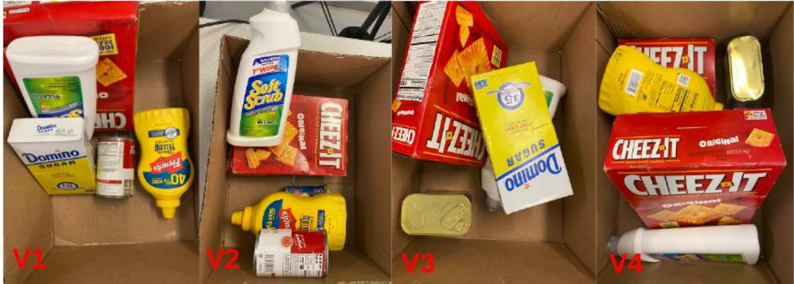
Figure 5.8: Example of failed packing executions, for each experimental condition. In the baseline (V1), all items are planned tightly, and the cracker box hit a container wall, causing it to tilt, and for all subsequent items planned on top of it to smash. In robust planning (V2), although margins were enforced in planning, a substantially incorrect pose estimation caused the bleach item to stick out of the container, and no action is taken to correct it. In closed-loop packing (V3), the first-placed cracker box caught on the side and failed to be pushed in. This was the only case when the push maneuver did not work in our examples. Although this caused a failed plan, replanning prevented the subsequent items from smashing onto the cracker box . With both closed-loop packing and robust planning (V4), a replan was triggered after the cracker box and before the bleach item. Because the pile was treated as a fixed, rigid object, the bleach was placed on top of the cracker box , but since it was unstable, this caused it to tip over.
