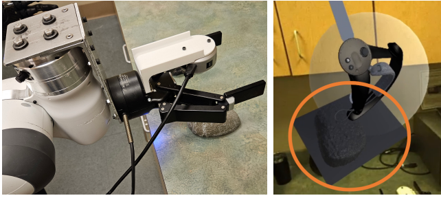
Fig. 2: A rock being scanned (left) and reconstructed as an AR mesh displayed in the headset (right). The operator can also “feel” the virtual object as the controller moves across it, as we map the reconstructed texture to vibrotactile and audio feedback.
